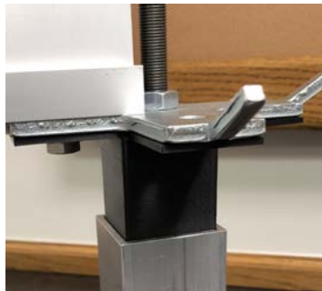
Bracket #2 attaches integrated post to the Polargy integrated ceiling. Bracket nests inside the post and has adjustable height of 4'
